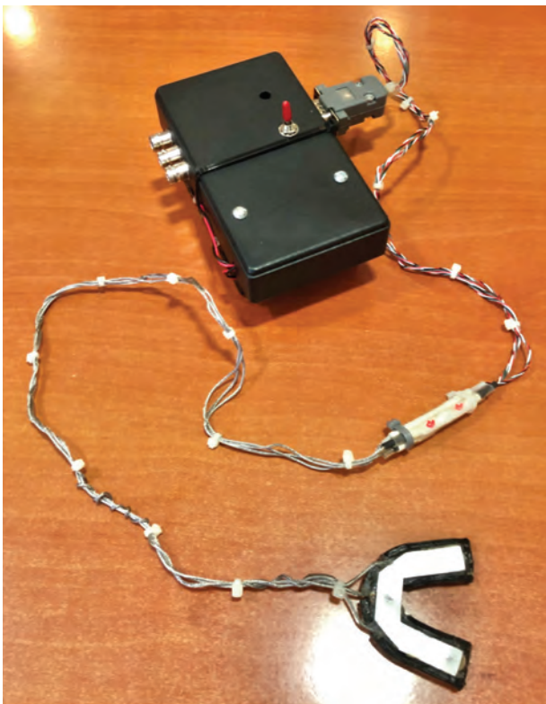
Figure 1. The dental apparatus of the bite force recorder device, designed to be suitable for the incisor and molar tooth sections, and the unit that amplifies the bite force data are shown
