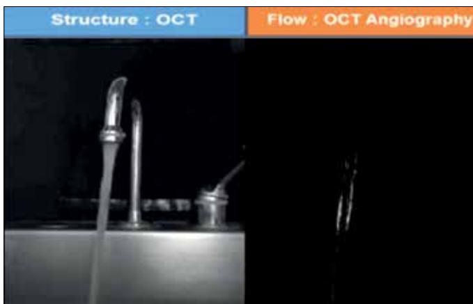
Figure 1. The basic principle of OCTA. Imaging of motion differences of two consecutive photo images digitally reproduces the image of water flow from a tap
