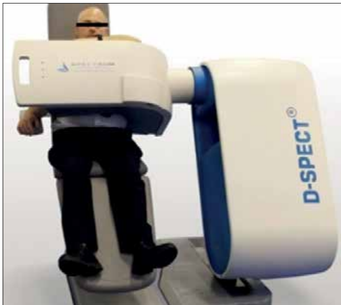
Figure 5. Spectrum Dynamics D-SPECT gamma camera with CZT detectors
