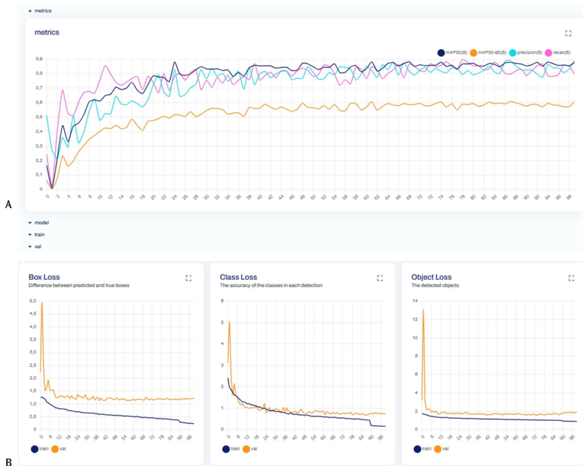
Figure 4. (A, B) Model accuracy measured on validation set, object loss, class loss, box loss graph during training of our model (Object loss measures the algorithm’s ability to correctly predict whether there are objects in an imagelabel. Class loss measures the algorithm’s ability to correctly guess which class objects in an image belong to. Box loss measures the algorithm’s ability to accurately predict the position and shape of objects in an image) (Ultralytics LLC, https://www.ultralytics.com/ )
